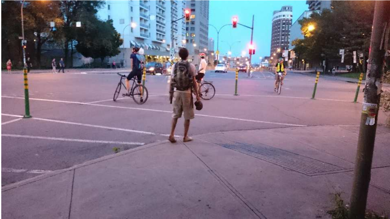
Above (Fig. 3) Intersection treatment is necessary and this can be piloted inexpensively with bump-out bollards at corners. These are removable during winter months if required and provide the added benefit of more pedestrian comfort. (Montreal)
